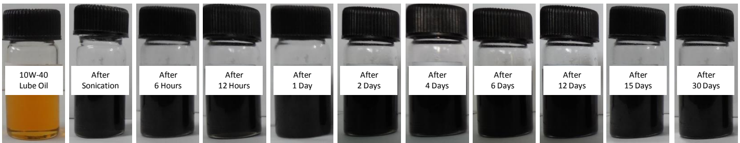
Dispersion of Chemically Functionalized Graphene in engine oil (Dose: 0.04 mg.mL -1 ) Till 30 days
