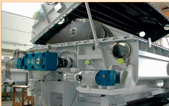
Filtration Section (Rotary Drum Filter)
