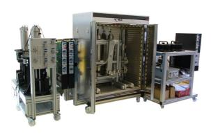
Purpose- Determine rock permeability and its interaction with various fluids
