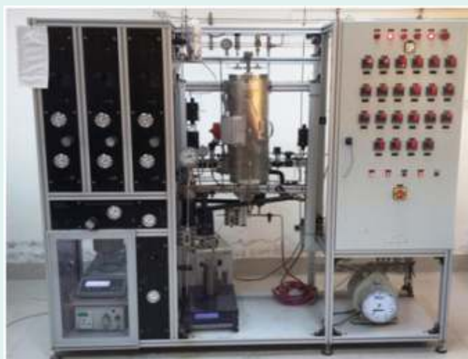
Reaction set-up used for the conversion of waste plastic naphtha to aromatics.
