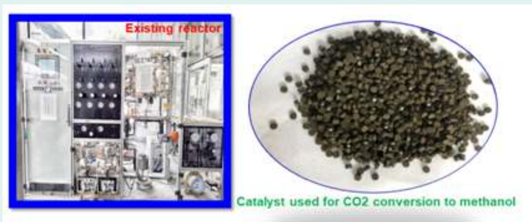
The Reactor used along with the Catalyst Developed for the CO 2 to Methanol Conversion
