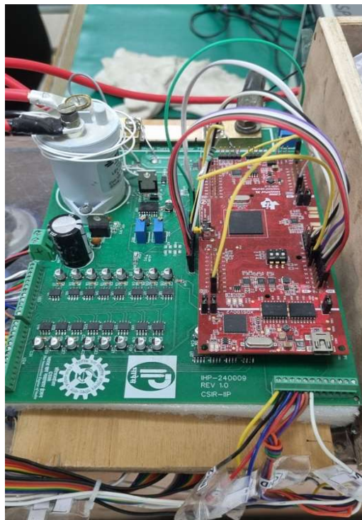
Fig. Final Assembled PCB Mounted on Supercapacitor Bank along with DSP
