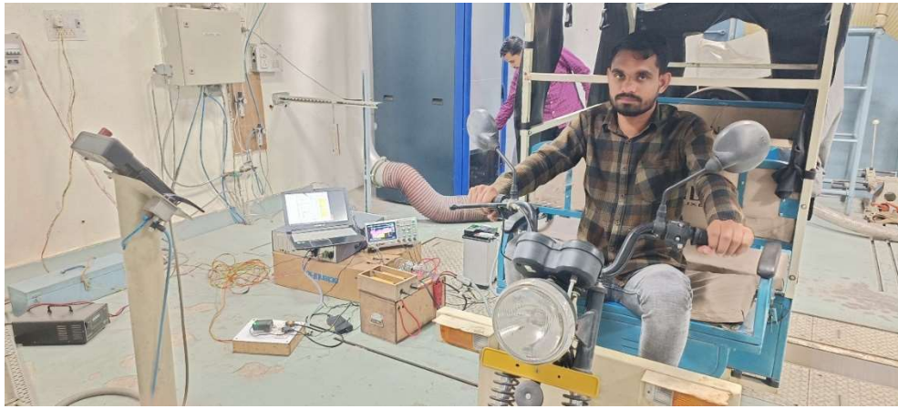
Fig. Dynamic Load Setup using 3-Wheeler E-Rickshaw
